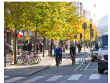
Götgatan has been redesigned with the help of removable bollards. This has enabled changes to be carried out quickly and designs to be tested before being made permanent.
